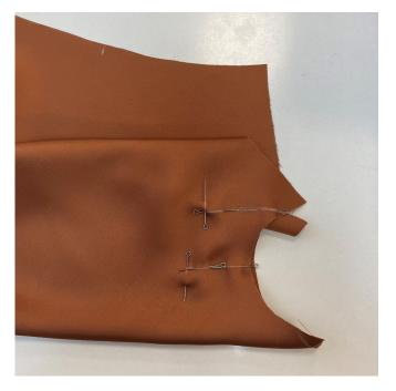
Pin and machine-stitch the pleats on the front bodice, backstitch at the beginning and end of each seam.
