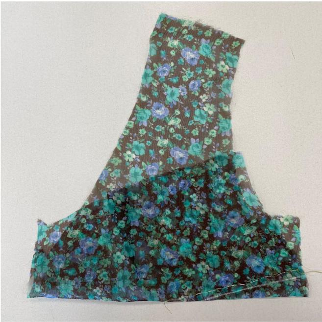
**Attention!** Darts, side and shoulder edges of the outer shell are finished with French seams. Finished dart and seam allowances are 5 mm (just under 1/4") wide.
